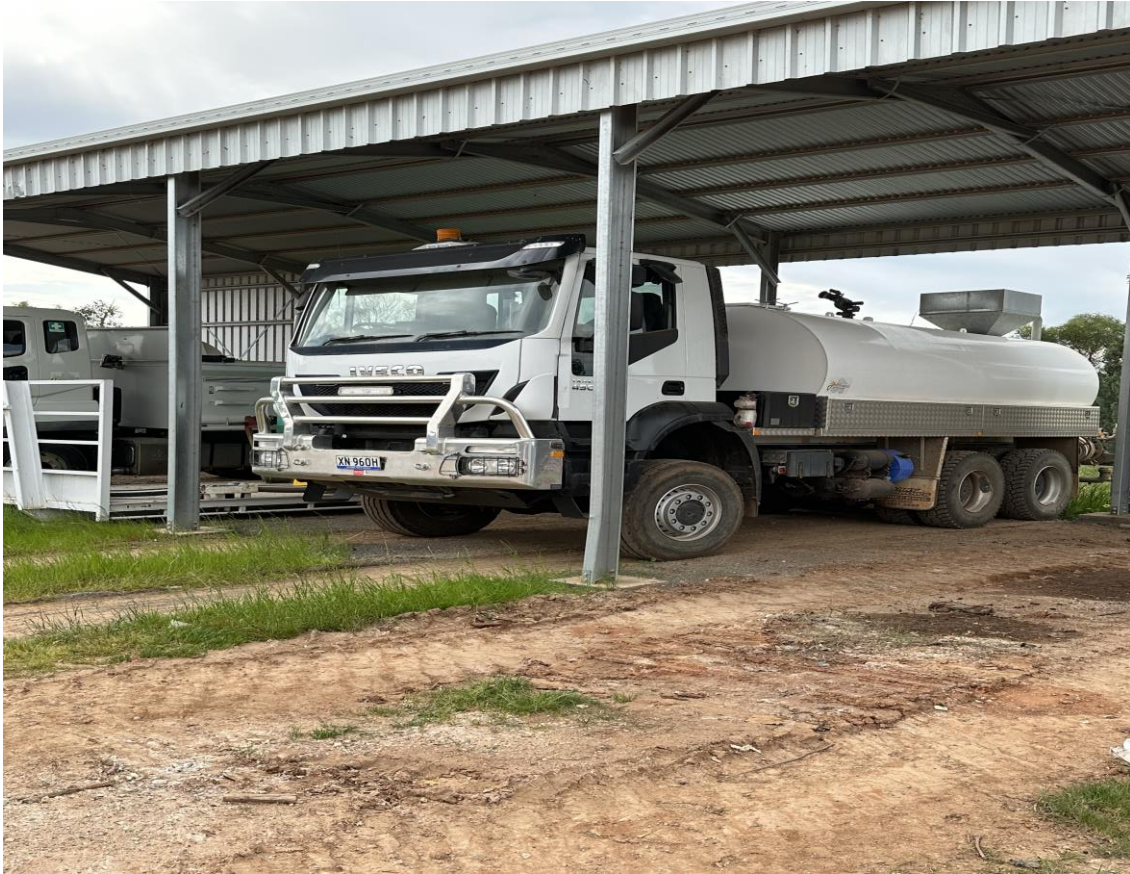
Water truck for fire and dust suppression
