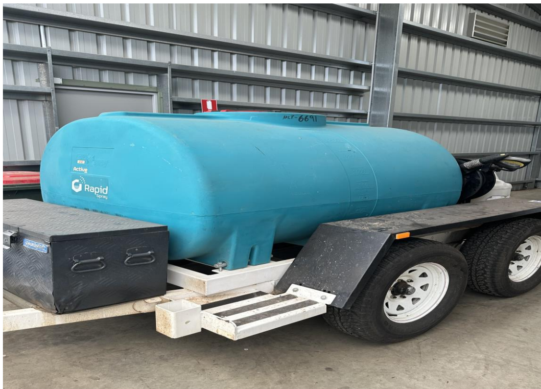
Water cart with sprayer for extinguishing fire and dust suppression
