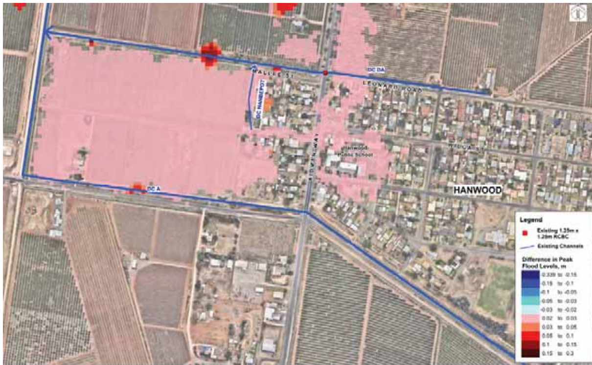
Figure 2-16 Difference Map for 1% AEP – TufLOW HPC vs TufLOW Classic
