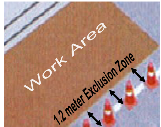
Example showing the minimum 1.2 meter separation distance between the work area and passing traffic
