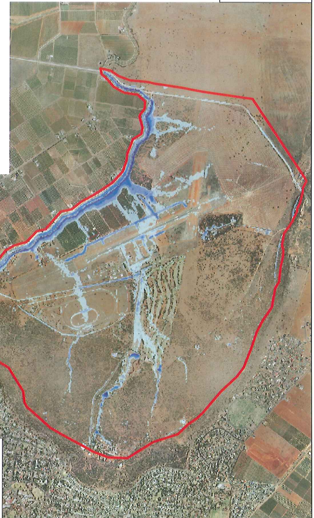
FIGURE 16 PEAK FLOOD DEPTH 2% AEP
