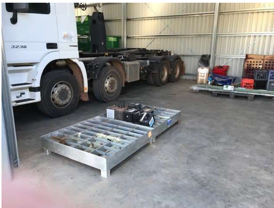
Figure 4.26: Bund for battery storage in the landfill workshop.
