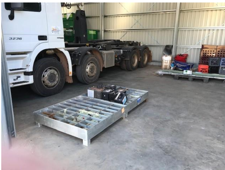
Figure 4.27: Bund for battery storage in the landfill workshop.
