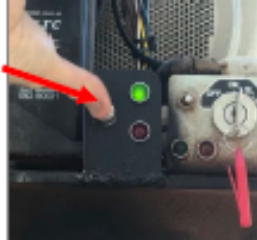
8 Reduce rev's by twisting throttle knob clockwise
