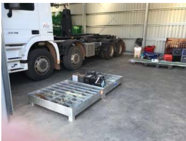
Figure 4.26: Bund for battery storage in the landfill workshop.
