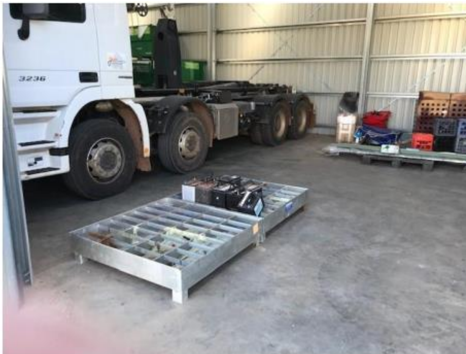
Figure 4-43: Bund for battery storage in the landfill workshop
